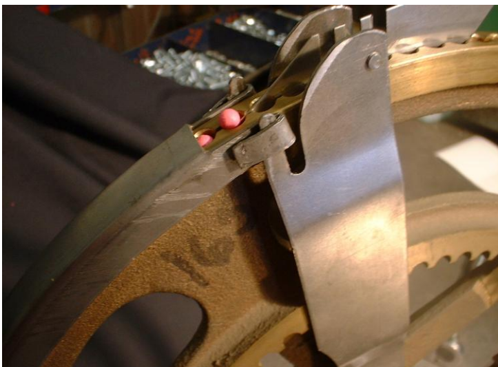
SEED WHEEL PROPERLY ADJUSTED
